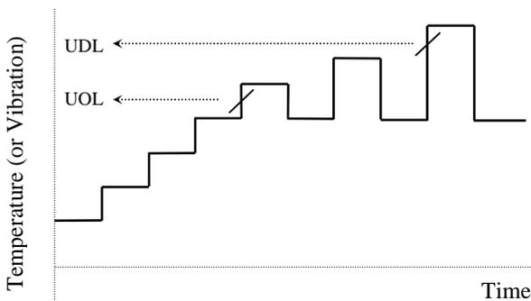
Figure 3 - Upper operational and destruct limits
