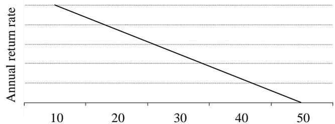
Figure 11 - Annual return rate vs operating margin ( °C)
