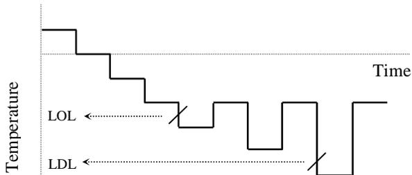
Figure 2 - Lower operational and destruct limits
