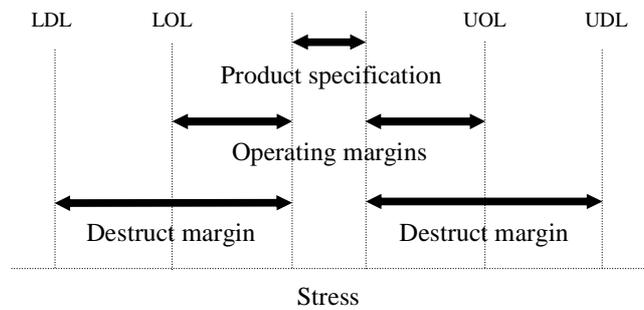
Figure 4 - Operating and destruct margins
