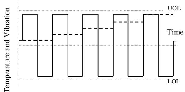
Figure 6 - Combined thermal cycling and vibration
