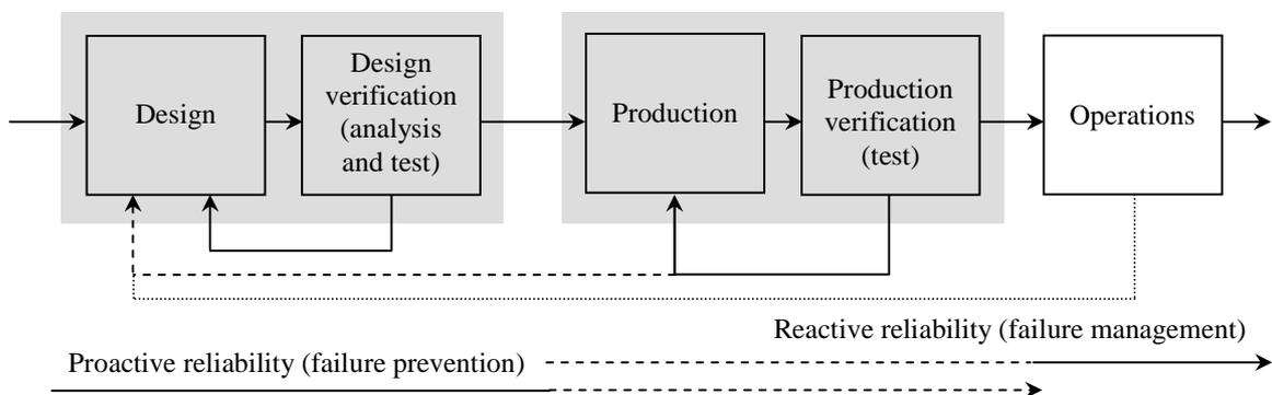
Figure 1 - Design and production verification
