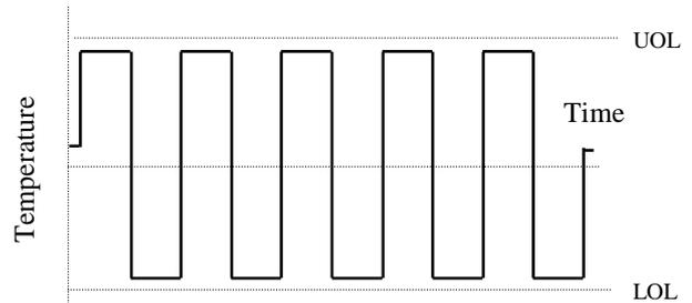
Figure 5 - Rapid thermal cycling
