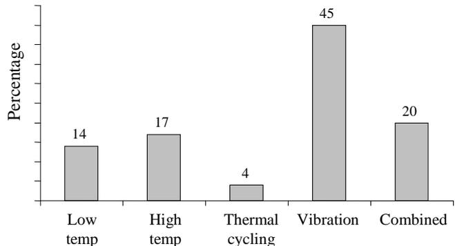
Figure 10 - Classical HALT failure modes observed
