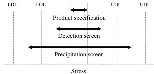
Figure 10 - Precipitation and detection screens
